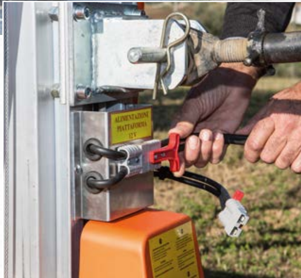
Powered by independent battery, or powered by 12V supply to the tractor.
